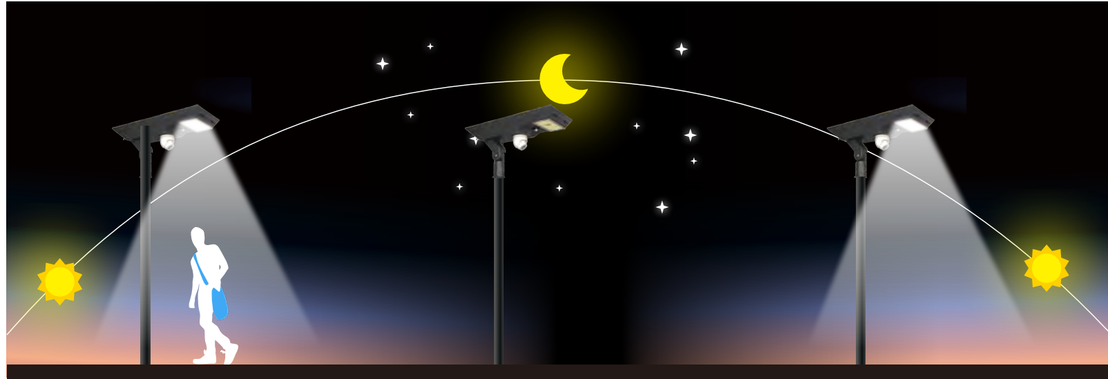
The motion sensor intelligent mode can remotely set the duration of 5 periods and the ratio of brightness with motion and without motion.
